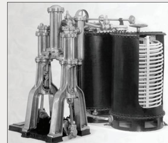
First Refrigeration Machine with Methyl Ether as the Refrigerant (*Courtesy of Linde North America, Inc.*)
