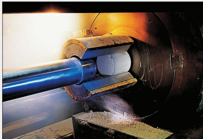
Aluminum Cylinder Extrusion
