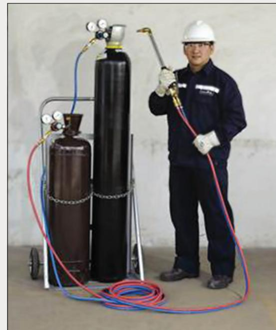
Modern Oxy Acetylene Welding Torch
