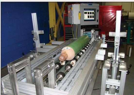
Ultrasonic Cylinder Testing Station
