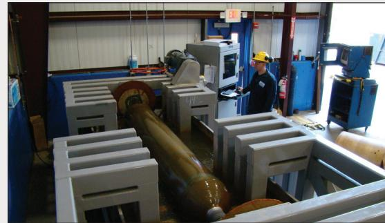
Ultrasonic Cylinder Testing (Courtesy of FIBA Technologies, Inc.)
